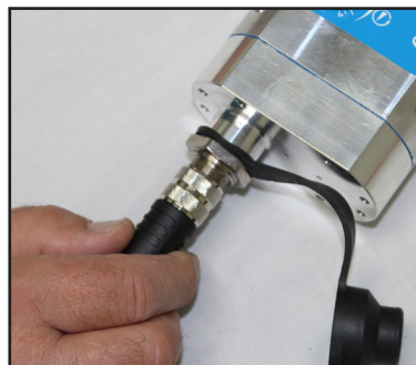
Figure 14. Attach Battery Pack Cable to Blower Unit
