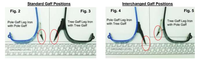
Gaff lengths when measured on the underside should not be less than 1-1/4" for pole gaffs or 2 1/4" for tree gaffs. When not being used for climbing, climber gaffs must be protected with gaff guards.
