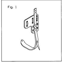
Attach sleeve to leg iron with sleeve loop facing outside of pad (away from the wearer's leg) using the fasteners enclosed. See Fig. 2 ('right' climber shown). <u>Note:</u> Two fasteners (screws, star washers & barrel nuts) must be used to secure each sleeve to each leg iron. Do not over tighten, torque to 25 inch pounds maximum.
